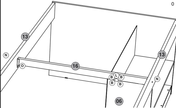
FIXE O SARRAFO CENTRAL (16) USANDO SUPORTE DE SARRAFO (O) E PARAFUSOS (N). FIXE A FACE DA DIVISÓRIA MENOR DIREITA (6) A FACE DO SARRAFO USANDO A CHAPINHA (L) E OS PARAFUSOS (B), COMO MOSTRADO NA IMAGEM.
